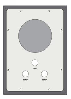
Figure 1: Experience Head One tube layout Never use excessive force when inserting the tubes into their socket.
