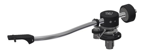
High-end 9-inch tonearm with fixed headshell for 1/2" hi-fi cartridge connection High-precision bearing technology with advanced tension compensating mechanism 246.75mm Effective mass: Effective length: 10.2g Offset angle: 22.25° Overhang: 16.75mm Outer null point: 120.9mm Inner null point: 66.04mm Connection: Hi-fi 1/2 inch Cartridge weight: 10...25g Output: Wire outlet 20cm 5-pin DIN outlet **Option DIN:**
