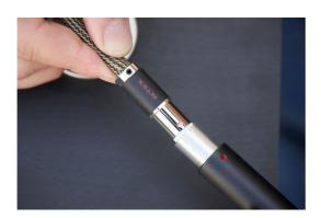
First fix the tonearm at medium height with a 1.5mm Allen key.
