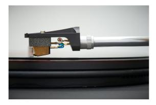
Personal preferences, such as setting the tone arm a little too high or too low, are welcome. In most cases, the height of the tonearm should be adjusted so that the cartridge and thus the edge of the headshell are parallel to the record surface.
