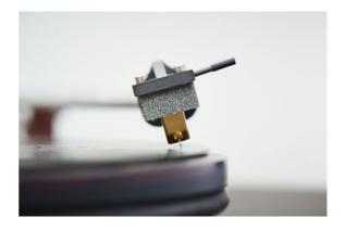
To illustrate, the azimuth is excessively misaligned.
