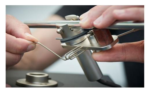
Slide on the anti-skating bracket from the side of the platter. Attention, the bracket must not touch the rotating part.
