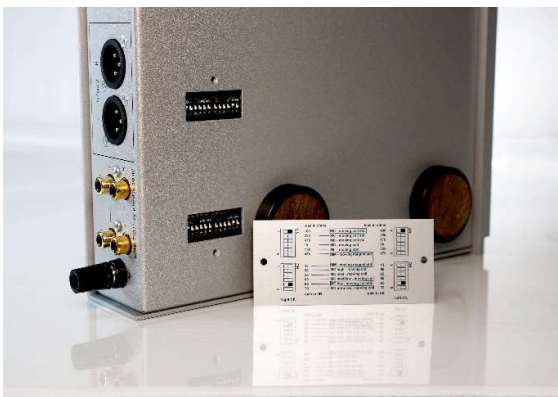
DIP Switch access with Aluminum locator plate
