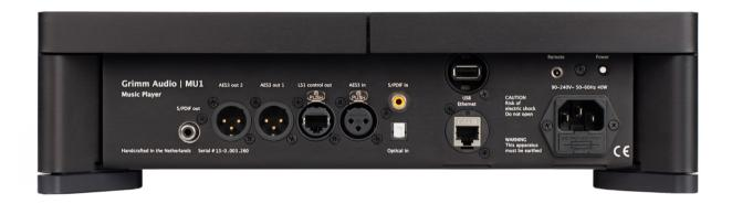
On the back of the MU1 you find, from left to right: four digital audio outputs (one generic S/PDIF, two generic AES3 and one Grimm LS1), three digital audio inputs, an ethernet network input, a USB connection for external storage, a 3.5mm socket for an external IR remote sensor, a small mains power switch and the mains power connector.
