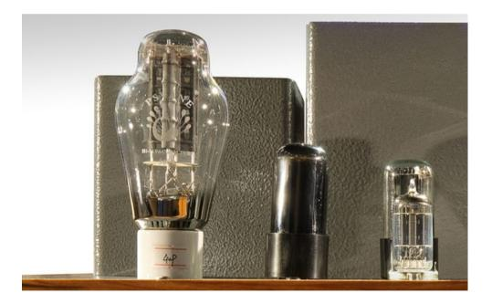
In the unit that was tested, all signal tubes are the so-called NOS, i.e. new (in the sense unused) tubes from old production. The circuit works, of course, in class A, without feedback. The amplifier is capable of delivering up to 7.5W of power per channel. It is heavy - it weighs 35 kg, which is not surprising, since one piece of the output transformer alone is 6 kg. For some users, it may be important to know that the manufacturer has prepared an appropriate tube cover for this amplifier.
